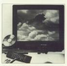
culture. As no keyboard is necessary, CDTV can be operated by people with no previous keyboard experience. CDTV exploits the technology of CD-ROM (compact disc read only memory) using discs with a storage capacity equivalent to around 720 floppy disks our about 250,000 pages of text.
